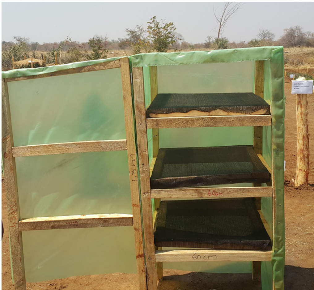
Figure 3.1 Solar drier made from plastic and wood
